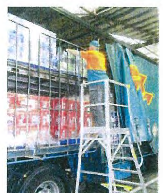
Using platform ladder to place angle guards and restraints
